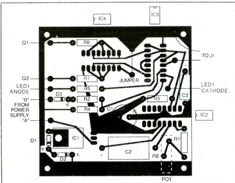
Fig. 4. Component-placement guide for pc board.
